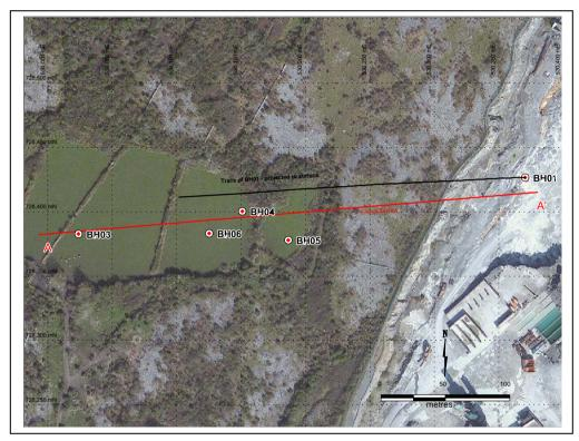
Figure 7: Borehole Collar Locations, Traces and Line of Section
